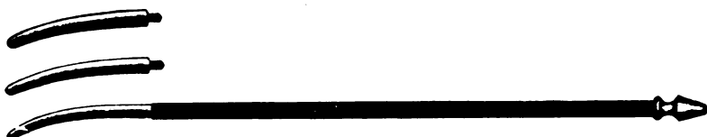
Fig. 241. Goelet's Intra-Uterin Negativ Dilating Electrode, nickel-plated, set of three bulbs with one staf. No. 115 McIntosh.
