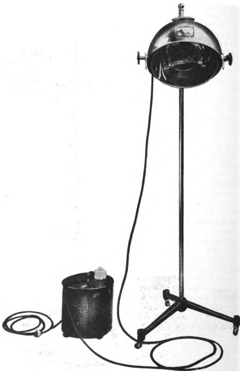
Fig. 177. Showing the Heraeus Alpine Sun, Quartz Mercury-Vapor Lamp for giving the air-cooled Quartz Light with an alternating current. M'd by Hanovia Chemical & Mfg. Co., Newark, N. J. The "drum" on the floor is a special transformer used with the alternating current. The burner used in this lamp is shown in Fig. 179.
