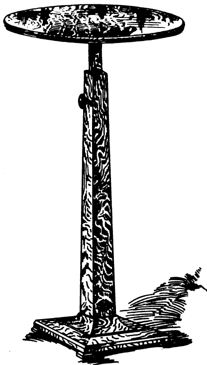
Fig. 120. Showing how a very attractiv offis or waiting-room table can be made to go on a Valens Adjustable Pedestal. Any good cabinet maker can make this elegant outfit. It should be made of quarterd oak, natural finish. The top is attacht to Pedestal by means of a Pedestal Pin.
