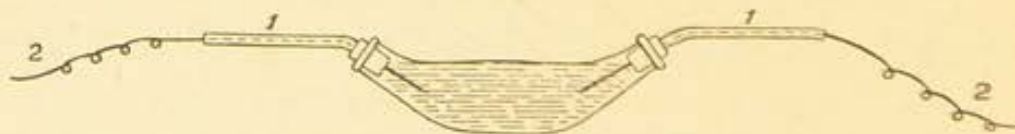
1 and 1 = contact wires. 2 and 2 = connecting wires to circuit shown in the next figure.
