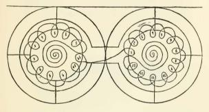
and fastened so that as it unwinds in one of the boxes it winds up the other in the second box. The clock is wound once a day, and as the running down of one of the spiral coils winds up the other the latter serves to run the clock during the night. Though it was described with much detail the mechanical working of it was not made clear, and hence we can only mention the ingenuity of the subconsciousness in constructing a plausible piece of machinery.
