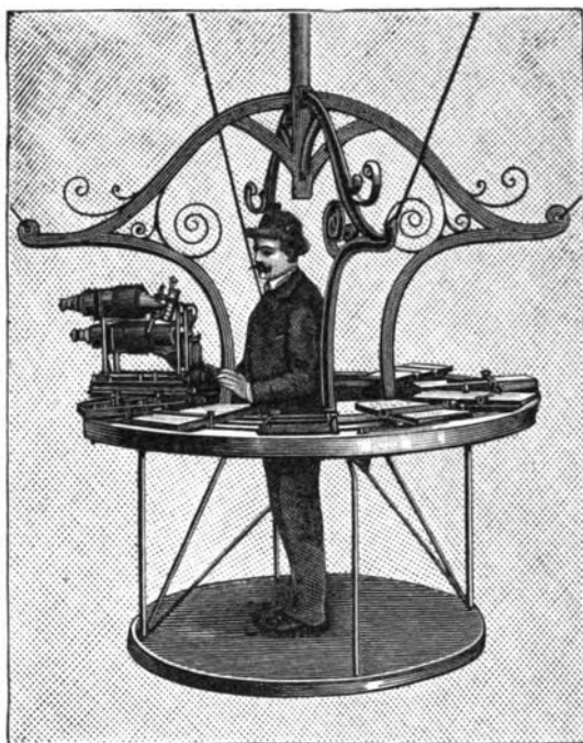
PLATFORM FOR THE OPERATOR AND PROJECTION APPARATUS SUSPENDED IN THE CENTER OF THE HALL.
