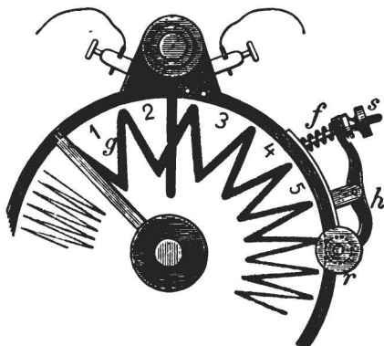
FIG. 4.—GRAPHITE RHEOSTAT, WITH MERCURY CONTACT.
