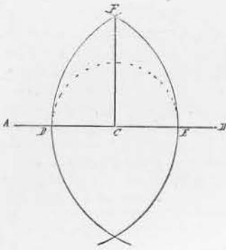
*Answer.*—From the given point C as centre describe an arc so as to cut the line A B in two points D and E. From the points D, E, with a radius equal to D E, describe arcs cutting each other at F, draw the straight line F C, then F C is perpendicular to A B and A C F is a right angle = to  $\square$ .
