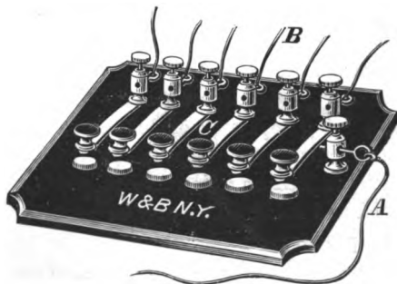
FIG. 35.—THE AUTHOR'S DIAGNOSTIC KEY-BOARD.— A , the rheophore which connects it with one of the binding-posts of a galvanic battery ; B , rheophores connecting its binding-posts with spring electrodes previously placed upon the body of the patient so as to influence the nerves or muscles to be tested ; C , buttons and springs which make a circuit to the body of the patient when the knob on the spring is pressed downward so as to impinge upon the button. The number of rheophores which may be employed depends upon the necessities of the case ; the cut shows an instrument capable of six.
