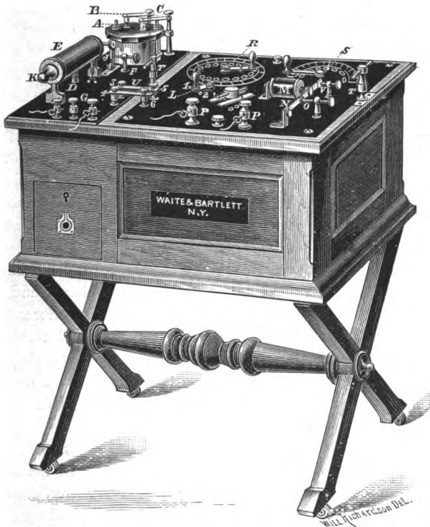
FIG. 27.—THE PHYSICIAN'S HANDY CABINET BATTERY.—The accompanying cut represents a light and compact form of cabinet battery, designed by the author. It is on castors, and can be wheeled about the consultation-room. This admits of the use of the instrument when the patient is in the gynaecological chair or upon the office lounge; or when any form of fixed apparatus, such as the laryngoscope, the inhaler or spray, etc., is being simultaneously employed. In some of my later models an immovable tray placed beneath the battery for electrodes, and a movable shelf is also provided upon which a milliamperè-meter, the solution of table salt, and the electrodes in actual use can be set. A glass cover protects the battery from dirt when not in use. E , faradaic coils; K , plunger; G , faradaic binding-posts; F , interrupter; D , drip-cup; R , current-selector of single cells; S , the same of four cells to each button; M , coil to work the interrupter for the galvanic current; L , switch to work or disconnect the interrupter ( V ); P , galvanic binding-posts; 3-5 and 4-6, connecting rods to allow of the action of M . The commutator lies above P .
