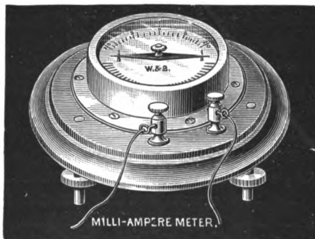
FIG. 19.—A HORIZONTAL MILLIAMPÈRE-METER (after the Thistleton pattern). The screw-feet allow of adjustment so as to insure a perfect leveling of the instrument. It is then revolved so that the needle (which will point north) rests at the zero point of the dial. Reversal of the current diverts the needle to the opposite side. One of the rheophores shown goes to a binding-post of the battery, and the other to one of the electrodes employed upon the patient. This instrument is very delicate, but the eye has to look down upon the dial in order to observe the deflection of the needle. If the instrument is placed lower than the eye, this objection is not serious. With it it is easy to detect small fractions of a millampère of current, and it is much less expensive than a good vertical galvanometer and more accurate than most of those offered to the profession.
