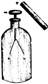
FIG. 7. ELECTROSCOPE. Ht. 12 in. Diam. 4\frac{1}{4} in.
