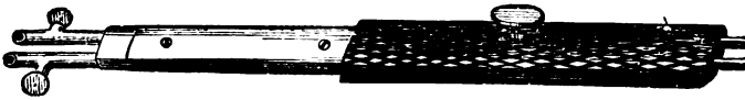
FIG. 26.—Handle for platinum knife or burner, with spring for closing and interrupting the circuit.
