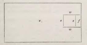
Let c represent the cistern, and the little square marked in it stand for the filter, to make which, lay up a box of brick, made
