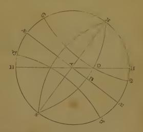
In the right angled spherical triangle DHN are given HN, the latitude of the place, and DN the complement of the declination, to find the angle DNH, which measured by the are BE, is the complement of the  $\Lambda$ D required; and in the angle  $\Upsilon$ BD, are given the angle B  $\Upsilon$ D = the colat, and BD the declination, to find  $\Upsilon$ B, the asc. diff.
