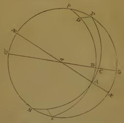
In the above diagram let A represent the position of a star in a northern sign with south latitude;  $\gamma$  B is its long, from  $\gamma$ . B A its latitude south, and C A it declination north. Then in the oblique angled spherical triangle A s S, are given  $\Lambda$  s = the complement of the star's lat.
