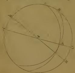
In the oblique spherical triangle ABC are given the angle ACB, the eo-longitude. AC the co-latitude, and AB the co-declination of the planet or star, to find its right ascension, viz. the co-angle at B.
