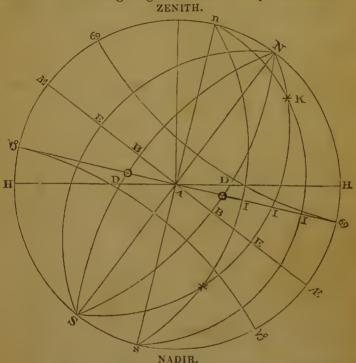
Construction.—With the chord of 60 degrees describe the circle Zenith H, Nadir H, and draw the diameter H H. Take the chord of 53 26, and set it from H to N; then
