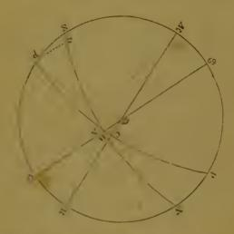
In this diagram A represents a star in a southern sign, with southern latitude also.  $\triangle$  B is its longitude, B A its lat. Then in the oblique angled spherical triangle A S p we have A S = the complement of its lat. p S, = the obliquity of the celiptic, with the angle p, S D = its longitudinal distance from the solstitial point  $\upmu$ . To find C A the star's declination. For which we have the following rules:—
