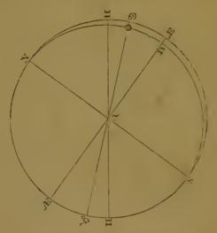
In the right angled spherical triangle A B  $\odot$ , A  $\odot = \odot$ 's longitude from the nearest equinoetial point, and the angle B A  $\odot = 23^{\circ}$  28' nearly,—the obliquity of the celiptic, are given to find B  $\odot$  = his present declination.
