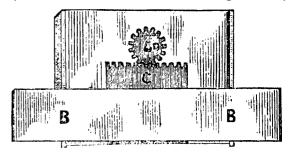
rack C gives motion to the wheel D, and the index points to the letters desired: the board BB works on small iron trucks having wood flats to keep the same in place.
