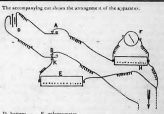
D, battery. F, galvanometer. H, shunt to cut off more or less of the current in order to regulate the deflec-on of the galvanometer. E, box of resistance coils. A and B, keys to make and break contact. (A) is always closed, and used only to correct or check zero. (B) pressed down to K, puts the resistance coils in place of the medium. The two wires on each side of the arrow go to the medium.
