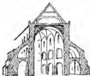
Later Romanesque, with concealed flying buttresses counteracting outward thrust of the vaulted roof.
