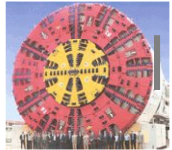
A Tunnel Boring Machine (TBM)
