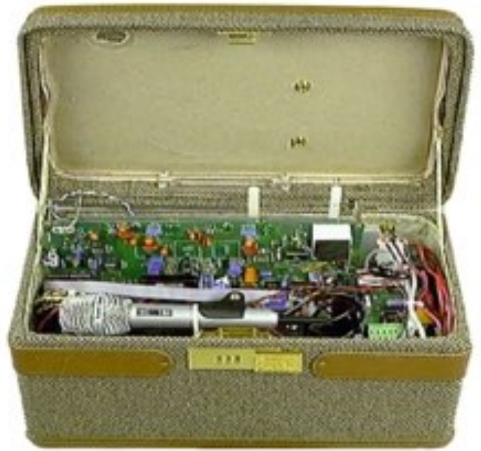
Figure 1. The URC AMP Project's first prototype, shown open. Batteries, power supply, and data logger are under the electronics board.
