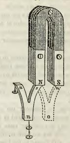
horse-shoe magnet, as seen in fig. 41, the lower end of the armature, and also the other branch of the fork acquire north polarity, and will sustain small pieces of iron. If both branches of the fork be applied, one to each pole of the magnet, as shown by the
