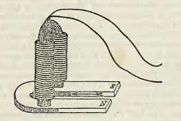
keeping each half applied to the same pole as before. Of course, the result will be the same, if the steel bar is kept stationary and the poles of the electromagnet passed over it in the proper direction of the arrow in fig 56.
