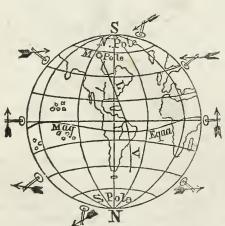
the needle makes with the horizon at any place, is called the dip, at that place. The tendency of the needle to dip is counteracted in the mariner's and surveyor's compasses, by making the south ends of needles intended to be used in northern latitudes, somewhat heavier than the north ends.
