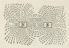
with the magnet in contact with its under surface, and then showering down iron sand or iron filings from a sand box held some inches above. The particles of iron, as they strike the paper can thus more readily assume the positions to which they tend un-
