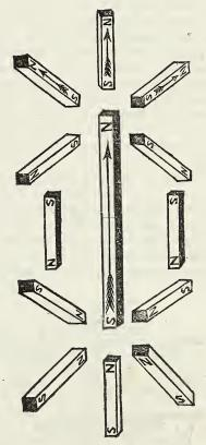
By passing such a needle carefully around a bar magnet, it will be found that it will assume positions in relation to it, as represented in the above cut.
