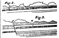
"Yet if a well be dug at any point, w, lower than that at which the porous stratum is exposed at the surface, water will rise in the same way as before.
