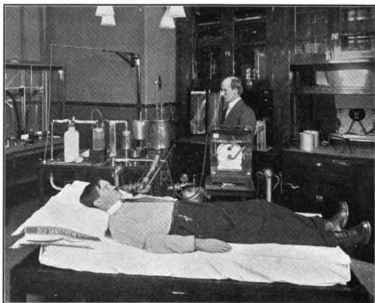
"Figure 1 shows the subject under test, lying on a couch breathing into and from the apparatus without, however, being confined in a chamber."
