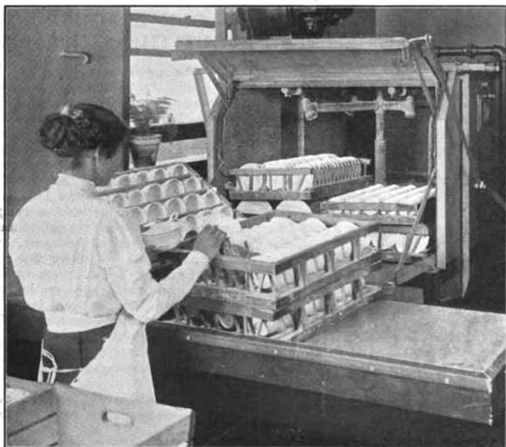
Neither pains nor money is spared to make every department of the Sanitarium as efficient as possible. To illustrate, the kitchen has just been supplied with the last word in dishwashers. The device holds four large trays of dishes. Hot water under pressure is directed on to the dishes from every direction, an important feature being the group of four rapidly revolving sprays, shown in the above picture. When the operation is completed the dishes are not only washed, but dried as well.
